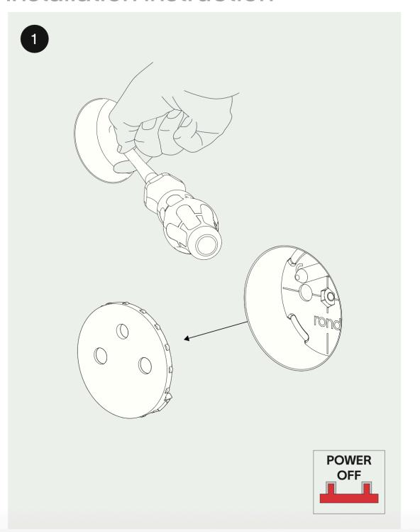
Gently remove the cover plate using a screwdriver. Place your finger between the screwdriver and the edge of the socket to prevent damaging the socket. Make sure the power is turned off before removal.
