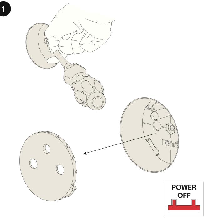
Gently remove the cover plate using a screwdriver. Place your finger between the screwdriver and the edge of the socket to prevent damaging the socket. Make sure the power is turned off before removal.
