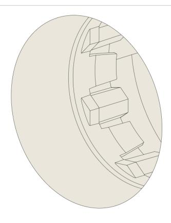
Remove the socket using the removal tool and follow the socket installation manual. The backfit holder is compatible with rond 3.0 retro / backfit / stone socket.
