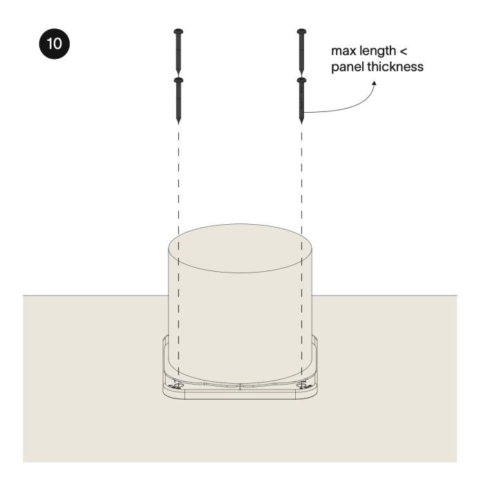
Fasten the backfit holder with junction box securely at the back of the material with the appropriate glue or screws on a screwfast surface.
