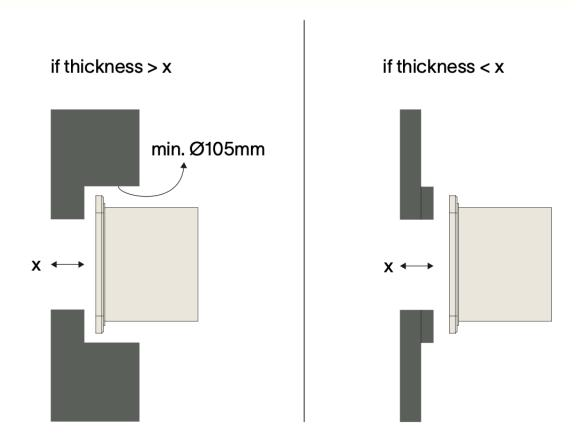
If the finish material thickness is not 19mm or 22mm (depending on choosen backfit holder), machine down or add (wooden) plate to achieve the correct total depth (19mm or 22mm).
