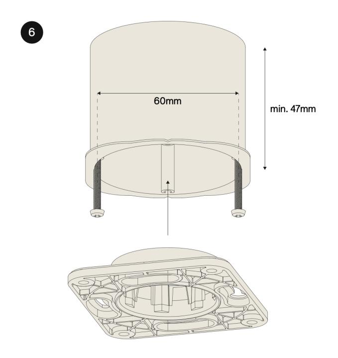
Install the backfit holder on the junction box.
